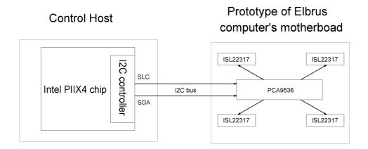
Fig. 2. Scheme of test bench
