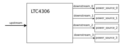
Fig. 4. Using LTC4306 multiplexer for accessing 4 power sources on target board
